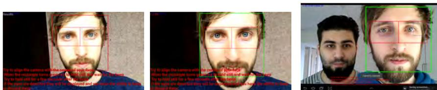
(a) Red layout on frame indicating incorrect ratio computed according to equation 1 (b) Green layout on frame indicating correct ratio computed according to equation 1 (c) Effectiveness of computed ratio to address multiple face in single frame
