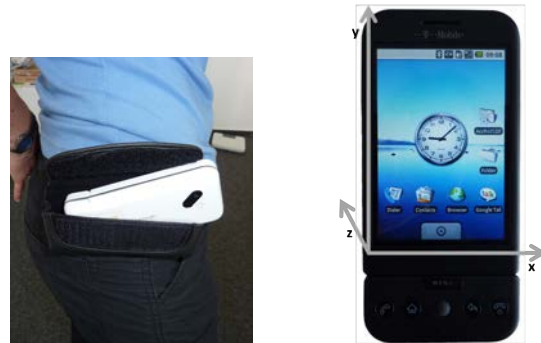
Figure 3. Phone attached to subject and the three axes in which acceleration is measured.
