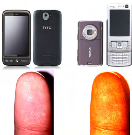
Figure 2. Left: CMOS Sensor (HTC Desire), Right: CMOS Sensor (Nokia N95) and a cropped/contrasted fingerprint image from each cell, at the same scale factor.
