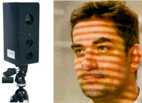
Figure 1: Capture device (left) and three-dimensional face scanning (right)
