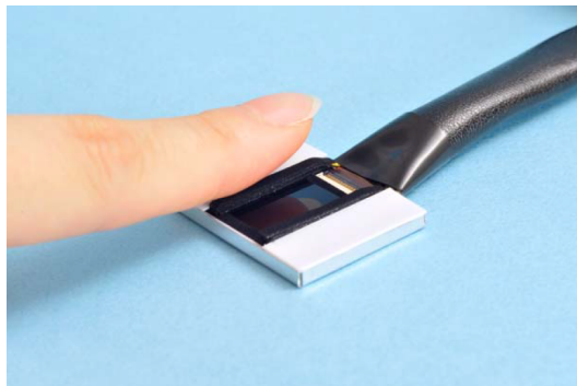
Figure 2.19: Miniaturized finger vein sensor from Hitachi (obtained from [89]).
